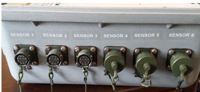
Figure 2. Left side socket connectors on the MM2 unit
