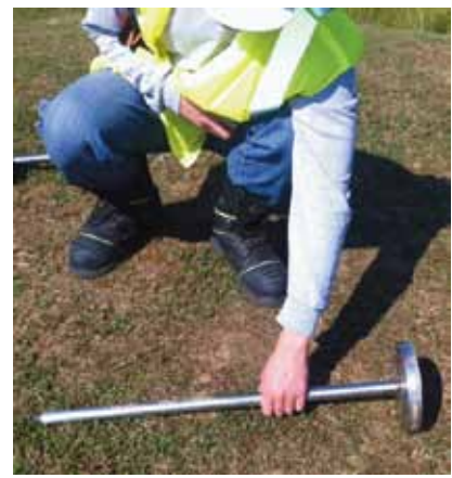
Figure 6. As an alternative to a hole, supplied spikes can be used.
