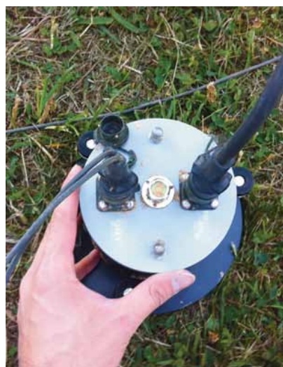
Figure 3. The sensors can be daisy chained to assist deployment.
