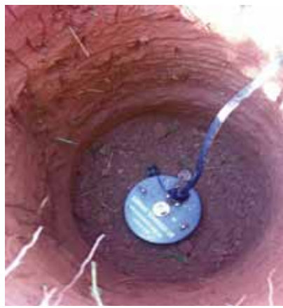
Figure 5. The sensor must be placed on solid earth.
