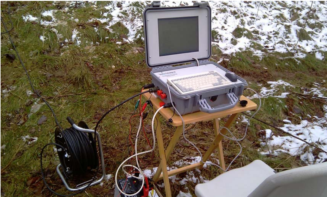
Figure 5. Photograph of the main processing unit, cabling and batteries.
