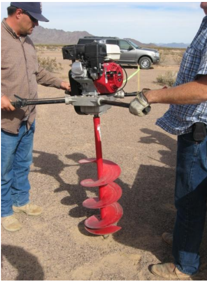
Figure 7: Example of a typical two man Auger being used to produce required holes.
