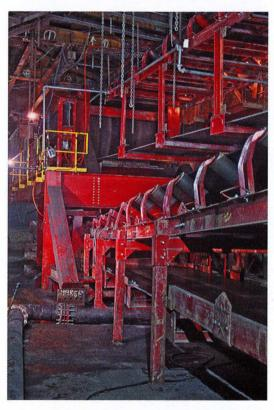
All of the surface conveyors at Sugar Camp Energy were also included in Joy's scope of supply. The surface conveyors include an 2,130 belt width raw coal stacker, a 1,520 mm plant feed conveyor, a 1,830 mm clean coal collecting conveyor and clean coal stacker conveyor, a 1,520 mm refuse collecting conveyor with 1,070 mm sub-refuse conveyors, and a 1,830 mm belt width train load out conveyor. All surface conveyors have been operating since May 2010.
